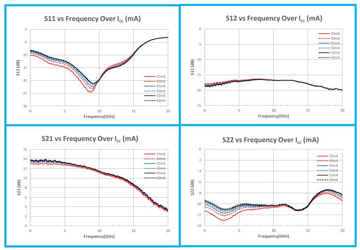
Note: The s-parameter gain results shown above were obtained using a micro-x package test fixture.
